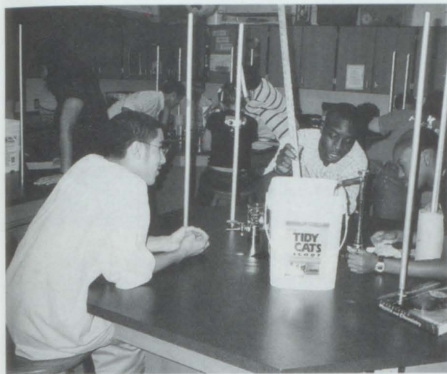
Robyn Reidel and Johnny Perez are measuring the length of water squirting out of the hole in the bucket.
