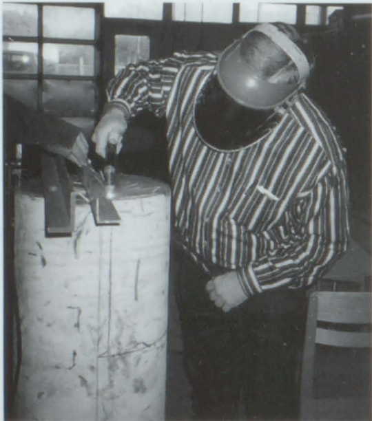
MR. USSERY USING A PLASMA CUTTER TO CUT THE DOOR ON THE BAR-B-Q PIT.
