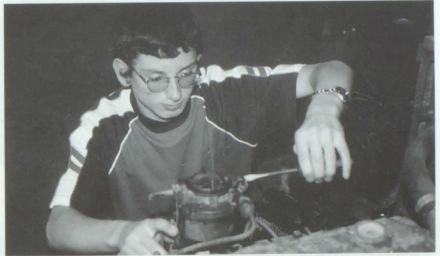
Above: Using a flat head screwdriver, Gerald Brietzke is work on adjusting a carburetor.
