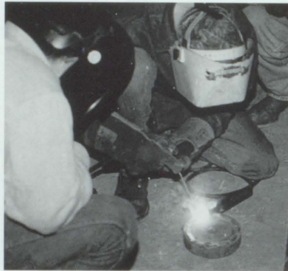
left to right:Daniel Hanzik building a trailer;Daniel Dykes welding coupons in the welding booth
