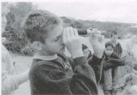
Justin Junek takes a salinity reading with a refractometer at the Intracoastal Waterway.
